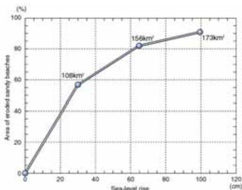
Another major problem is the erosion of sandy coastlines. While the main causes of erosion are a decreasing sediment supply and block of longshore sand transport, sea level rise will accelerate beach erosion. If the sea level rises 30 cm, it is estimated that at least 56.6% of the sand beaches in Japan will be eroded (Figure 5). If the sea level rises 65 cm to 1 m, sand beach erosion will reach as much as 81.7% to 90.3%.
